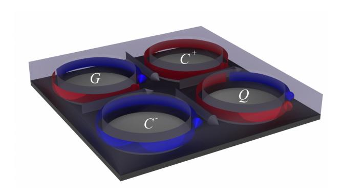
Researchers at the Helmholtz Zentrum Dresden-Rossendorf in Germany have calculated that the specific layout of four holes ("antidots") in a layer of cobalt will accommodate 15 different combinations for programming. Credit: HZDR
