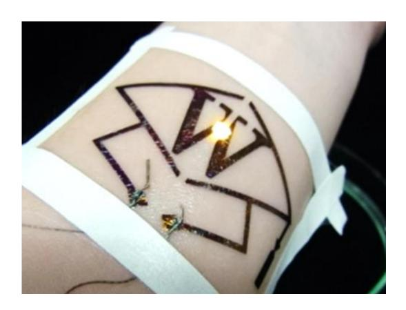
A sandwich of printed circuits and SBS elastomer is just 750 nm thick, for extremely high flexibility and comfort. Credit: Waseda University
