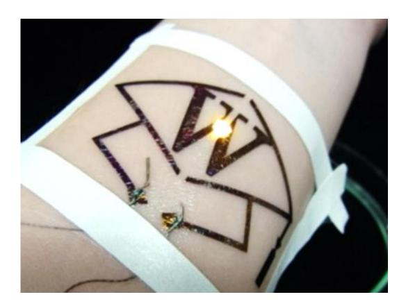
A sandwich of printed circuits and SBS elastomer is just 750 nm thick, for extremely high flexibility and comfort. Credit: Waseda University
