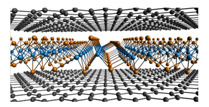
A ball and stick model of the graphene-tungsten ditelluride-graphene stack used for imaging in the research. Credit: University of Pennsylvania
