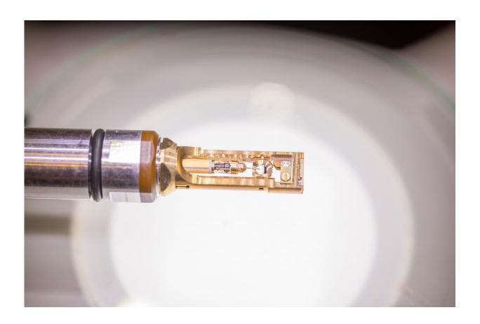
Researchers performed imaging and resistance measurements in a transmission electron microscope using a sample holder with a nanoscale electrical probe. Credit: Mikko Raskinen / Aalto University
