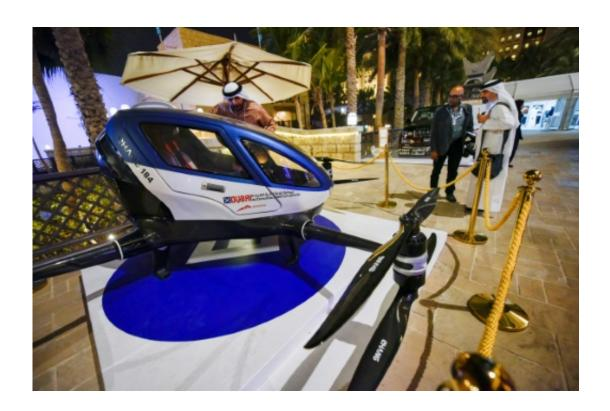
The electric EHang 184 can travel at 100km per hour at 300m above the ground, the Dubai transport authority says
