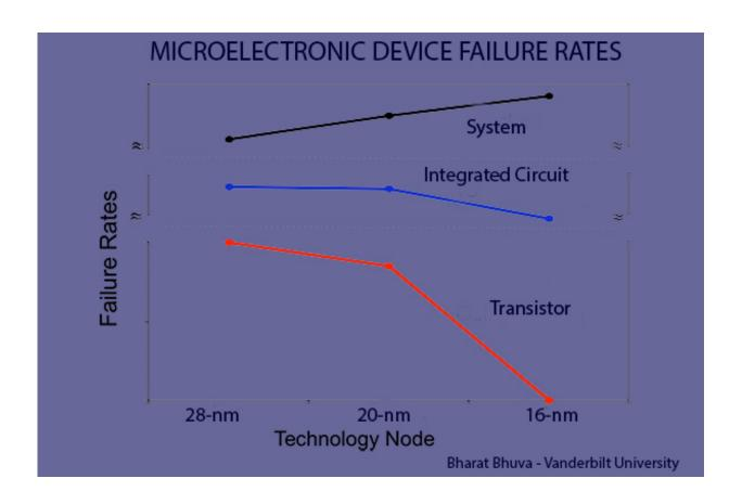
Estimated failure rates from single event upsets at the transistor, integrated circuit and device level for the last three semiconductor architectures. Credit: Bharat Bhuva, Vanderbilt University
