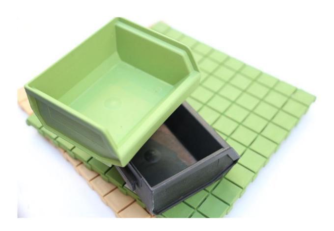
Up to half of oil-based polypropylene can be replaced with paper industry side streams. Plastec Finland Oy and Wiitta Oy made a trial batch of floor tiles and storage containers, of which side-streams accounted for 30%.
