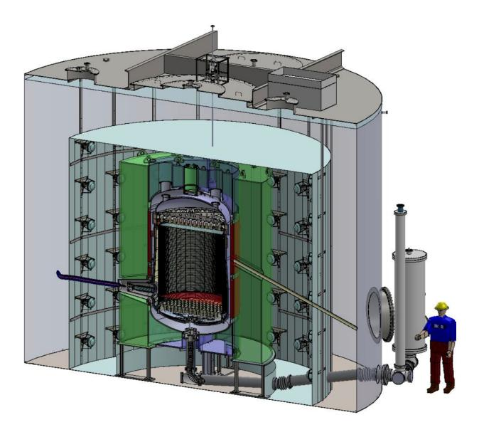
A cutaway rendering of the LUX-ZEPLIN (LZ) detector that will search for dark matter nearly a mile below ground. An array of detectors, known as photomultiplier tubes, at the top and bottom of the liquid xenon tank are designed to pick up particle signals. Credit: Matt Hoff/Berkeley Lab
