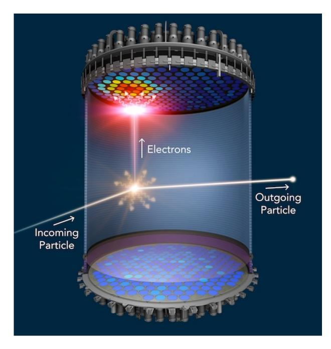
Inside LZ: When a theorized dark matter particle known as a WIMP collides with a xenon atom, the xenon atom emits a flash of light (gold) and electrons. The flash of light is detected at the top and bottom of the liquid xenon chamber. An electric field pushes the electrons to the top of the chamber, where they generate a second flash of light (red). Credit: SLAC National Accelerator Laboratory
