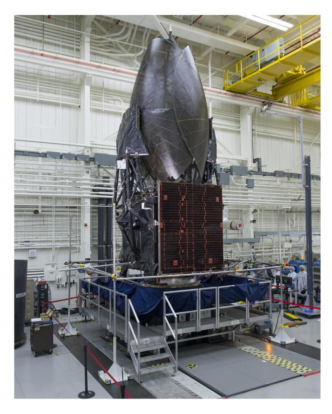
TDRS-M undergoes vibration testing. Credit: Boeing
