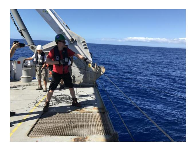
NASA scientist Ryan Vandermeulen deploys a set of profiling radiometers to measure ocean color. Credit: NASA's Goddard Space Flight Center/Stephanie Schollaert Uz
