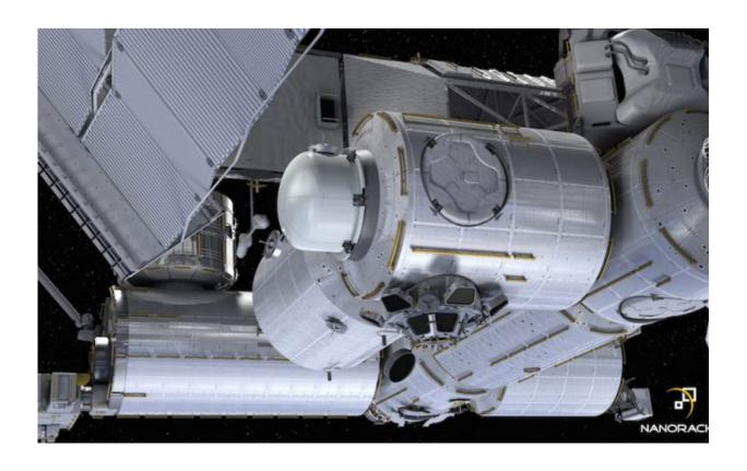
Artists concept of first commercially funded airlock on the space station being developed by NanoRacks that will launch on a commercial resupply mission in 2019. It will be installed on the station's Tranquility module. Credit: NanoRacks
