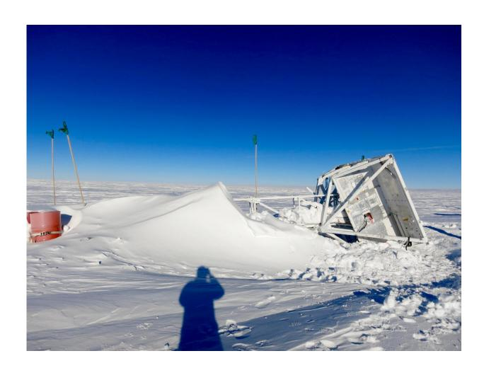
The GRIPS telescope parachuted to the ground and sat on the ice for an entire year. Scientists had to dig out snow to recover the GRIPS instruments, but not much snow made it into the electronics themselves. Credit: Hazel Bain, University of California, Berkeley
