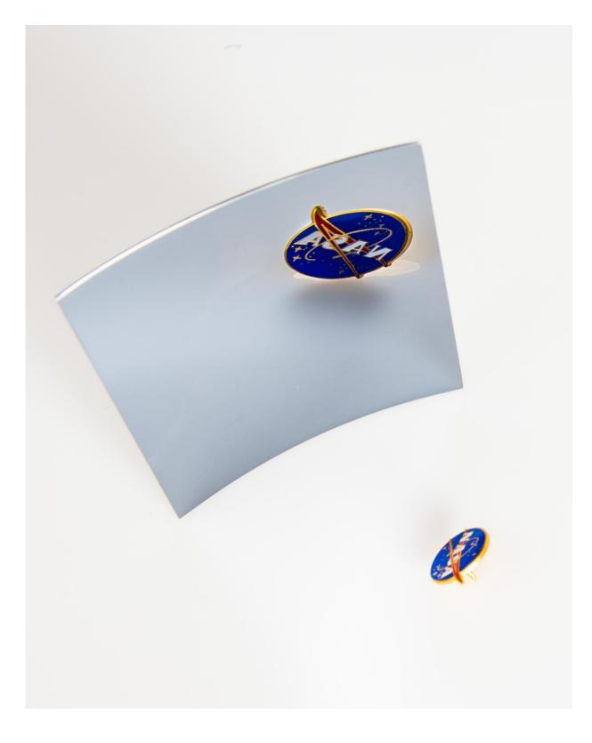
Thin, lightweight, high-resolution mirrors, such as the one shown here, are vital to next-generation X-ray missions. Will Zhang and Raul Rivera are advancing a
