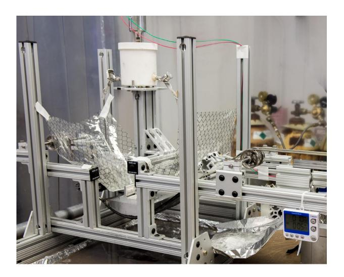
Scientist Will Zhang has created a manufacturing facility to create a new-fangled X-ray optic made of silicon. This image shows the buffing machine to remove imperfections from the mirror's surface. Credit: NASA/W. Hrybyk
