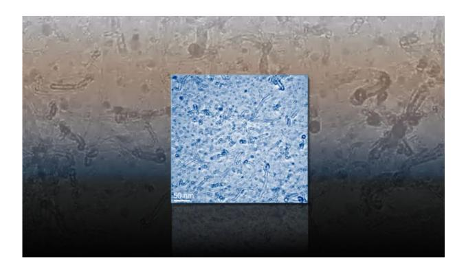
This transmission electron microscope image shows growth of a dense carbon nanotube population. Credit: Lawrence Livermore National Laboratory
