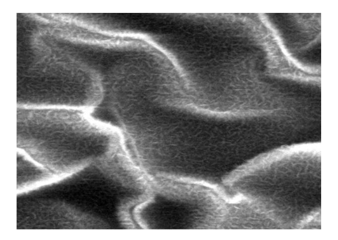
Scanning electron microscope image of atomically-thin MoS2 with hierarchical, dual-scale structures. Credit: SungWoo Nam, University of Illinois
