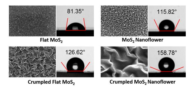
Images of atomically thin MoS2 with micro- and nano-scale roughnesses and their corresponding water contact angles. Credit: SungWoo Nam, University of Illinois
