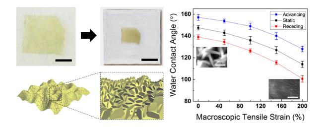
Image shows how controlled and dynamic surface architecturing/roughening of atomically thin MoS2 affects wettability. Credit: SungWoo Nam, University of Illinois
