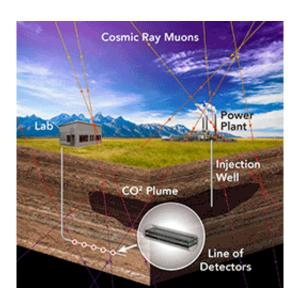
In this illustration, a series of five borehole muon detectors are deployed in a horizontal well below a carbon dioxide reservoir. Credit: Pacific Northwest National Laboratory
