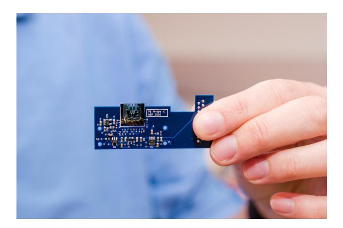
A MEMS-based atomic force microscope developed by engineers at the University of Texas at Dallas is about 1 square centimeter in size (top center). Here it is attached to a small printed circuit board that contains circuitry, sensors and other miniaturized components that control the movement and other aspects of the device. Credit: University of Texas at Dallas
