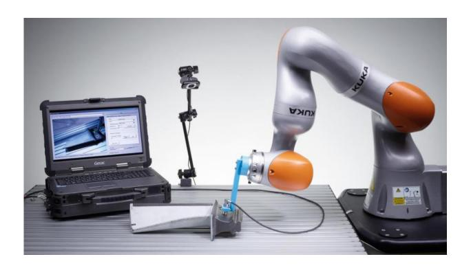
AR-system for intelligent inspection and quality control of safety-critical objects. Credit: Fraunhofer IZFP
