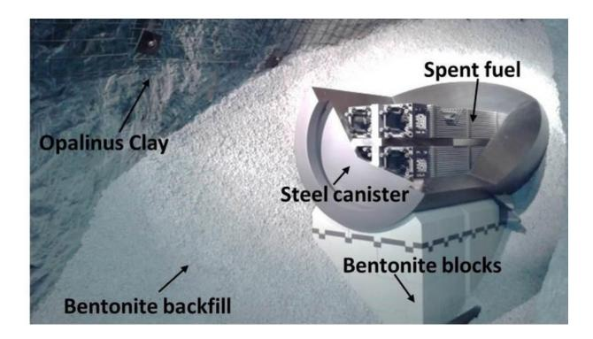
Model of a storage tunnel for used fuel elements. Credit: LMS/EPFL, Mont Terri underground lab
