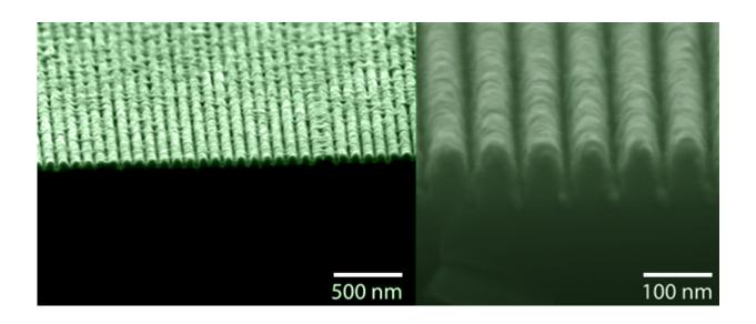
SEM images of a 'lossless' metamaterial that behaves simultaneously as a metal and a semiconductor. Credit: Ultrafast and Nanoscale Optics Group at UC San Diego
