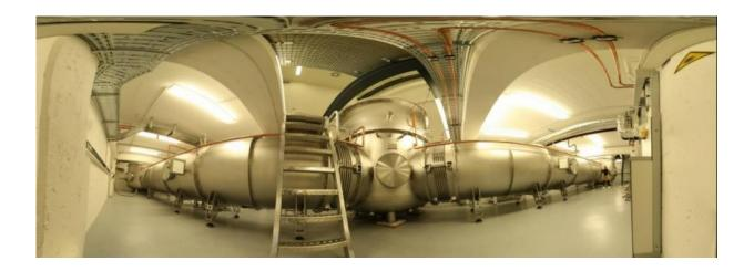
Panorama shot of the 10 meter prototype at the Max Planck Institute for Gravitational Physics in Hannover. It is used for demonstrations and tests of technologies for the third generation of gravitational-wave detectors. Credit: Lück/Max Planck Institute for Gravitational Physics
