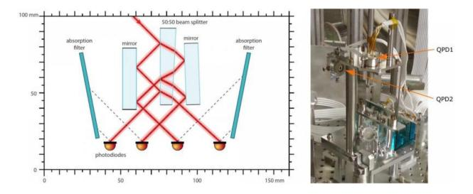
he photodetector system used for the power stabilization. Left: schematic of the beam path of the laser (red) onto the four measurement photo diodes via mirrors. Right: The device being integrated into the AEI 10 meter prototype. The four measurement photo diodes are on the right backside. The additional photodiodes for stabilization of the beam pointing are on the top, marked QPD1/2. Credit: Junker/Kwee/Max Planck Institute for Gravitational Physics
