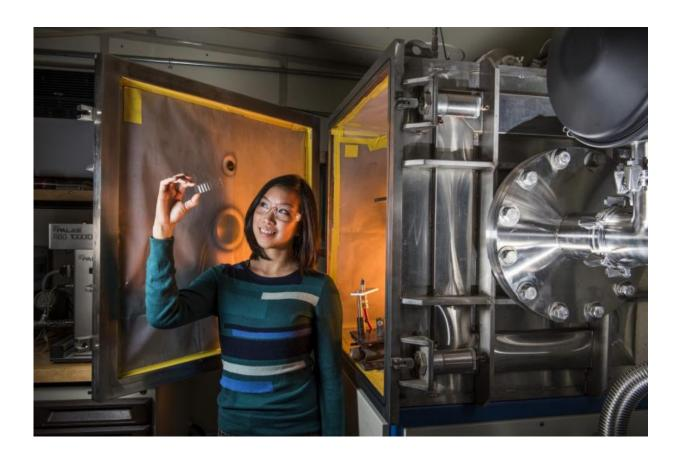
Sandia National Laboratories researcher Pylin Sarobol looks at samples of carbide coatings as she stands in front of a deposition chamber. Sarobol and colleagues are working on a process to lay down ceramic coatings kinetically, avoiding the high temperatures that otherwise would be required. Credit: Randy Montoya
