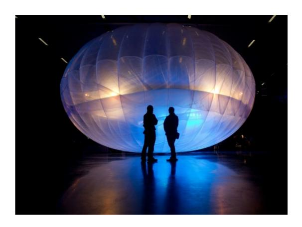
"Project Loon" uses roaming balloons to beam internet coverage to remote areas outside the range of ground-based telecommunication towers
