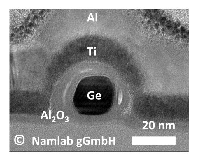
Energy-efficient germanium nanowire transistor with programmable p- and nconduction is shown. Transmission electron microscope image of cross section. Credit: NaMLab gGmbH
