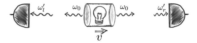
The friction-like change in momentum discovered in the new study can be modeled by a moving device that emits photons in opposite directions. An observer can measure the photon frequencies, and using the Doppler effect, will calculate a change in momentum but no change in velocity. Credit: Sonnleitner et al. ©2017 American Physical Society
