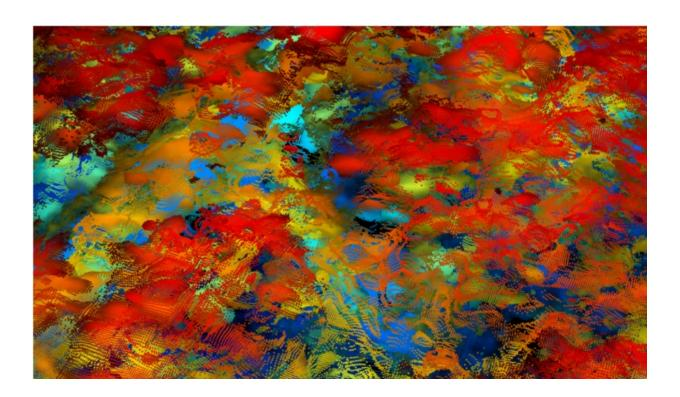
This example of a 3-D ladar point cloud shows a fully foliated field site. Color indicates elevation above the ground, with red tones indicating a higher elevation value (for example, tree tops and vegetation) and blue tones indicating lower elevation value (ground-level vegetation and the ground itself). Credit: Massachusetts Institute of Technology
