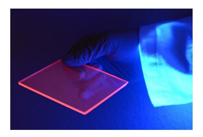
While most of the light concentrated to the edge of the silicon-based luminescent solar concentrator is actually invisible, we can better see the concentration effect by the naked eye when the slab is illuminated by a "black light" which is composed of mostly ultraviolet wavelengths. Credit: Uwe Kortshagen, College of Science and Engineering
