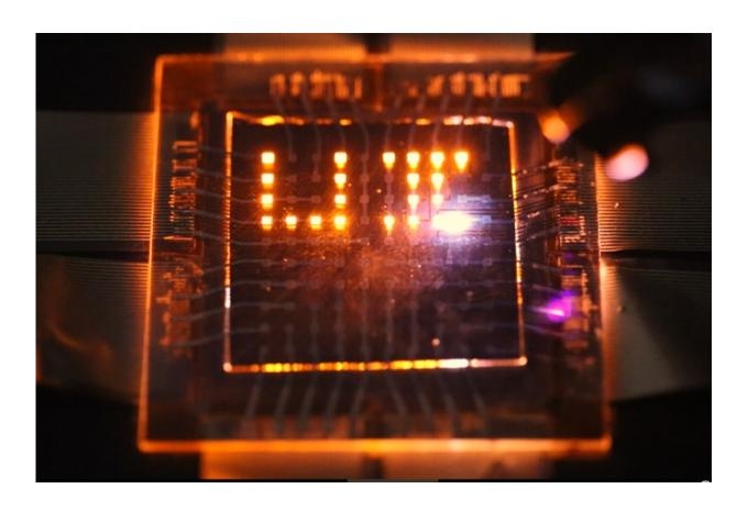
A laser stylus writes on a small array of multifunction pixels made by dualfunction LEDs than can both emit and respond to light. Credit: Moonsub Shim, University of Illinois
