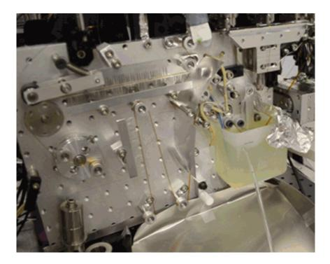
Droplet-on-tape conveyor belt system delivers samples at the Linac Coherent Light Source (LCLS). Credit: SLAC National Accelerator Laboratory
