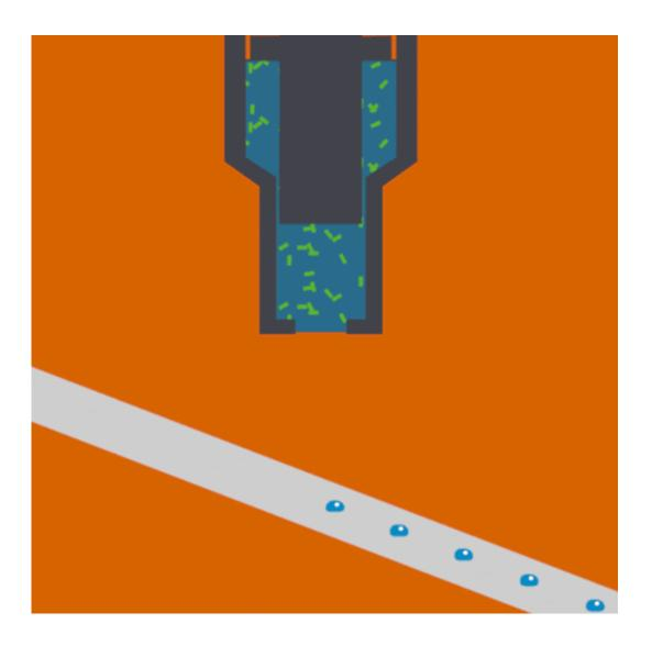
Acoustic droplet ejection allows scientists to deposit nanoliters of sample directly into the X-ray beam, considerably increasing the efficiency of sample consumption. A femtosecond pulse from an X-ray free-electron laser then intersects with a droplet that contains protein crystals. Credit: SLAC National
