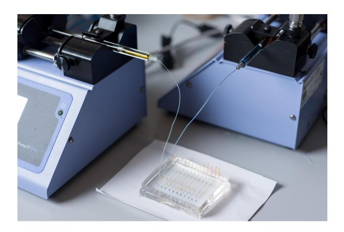
A microfluidic chip used to fabricate nanoparticles that could be used to deliver therapeutic genes to specific organs of the body. Credit: Rob Felt, Georgia Tech
