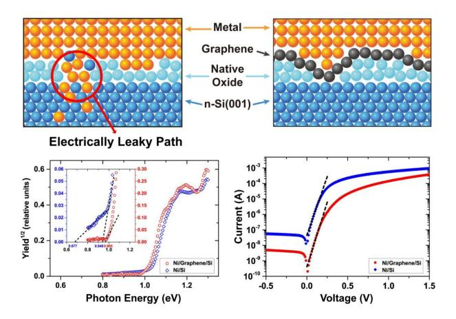
The schematic view of internal photoemission (IPE) measurements on metal/n-Si(001) junctions with Ni, Pt, and Ti electrodes for with and without a graphene insertion layer. Credit: Ulsan National Institute of Science and Technology
