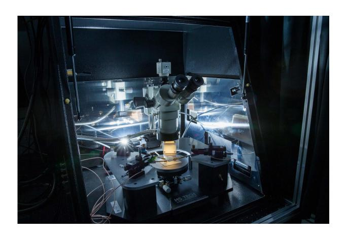
Shown above is the Internal Photoemission (IPE) Measurement System, developed by Hoon Hahn Yoon, combined M.S./Ph.D. student of Natural Science at UNIST. Credit: UNIST
