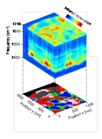
Nanoscale-resolved hyperspectral infrared data cube of a polymer blend, comprising 5000 nano-FTIR spectra (top panel). The data cube can be divided into clusters (by hierarchical cluster analysis) and thus converted into a compositional map (bottom panel). It reveals the polymer components (grey, blue and red areas), as well as the interfaces between them (green areas) that partially exhibit anomalies that are explained by chemical interaction (purple areas). Credit: CIC nanoGUNE
