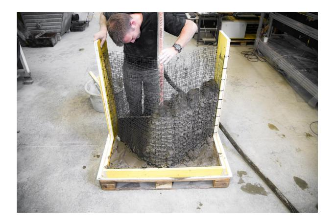
Mesh Mould prototype produced by In Situ Fabricator construction robot is being filled with concrete. Credit: NCCR Digital Fabrication and ETH Zurich
