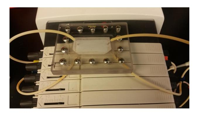
This reusable, multi-layered and microfluidic device incorporates a porous growth substrate, with a physiological fluid flow, and the passive filtration of the capillaries around the end of a kidney, called the glomerulus, where waste is filtered from blood. Credit: Gretchen Mahler
