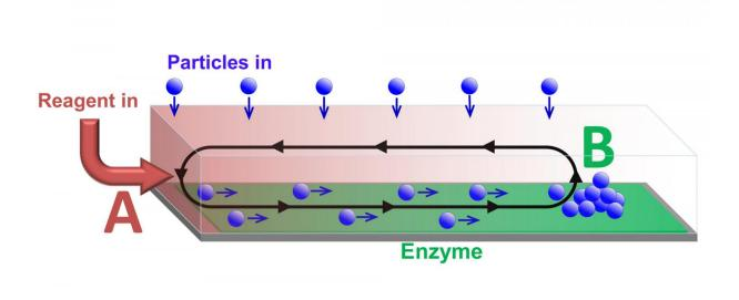
Particles transported along a channel by chemically-driven fluid flow. The flow is generated by reagent entering at one end of the channel (A) and reacting at the enzyme covered surface. The cargo is deposited at position B, which can be controlled by varying the reaction rate. Credit: Oleg E. Shklyaev and Henry Shum
