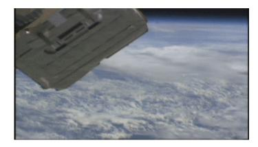
CubeSats are deployed into orbit from the NanoRacks module aboard the International Space Station. Credit: NASA
