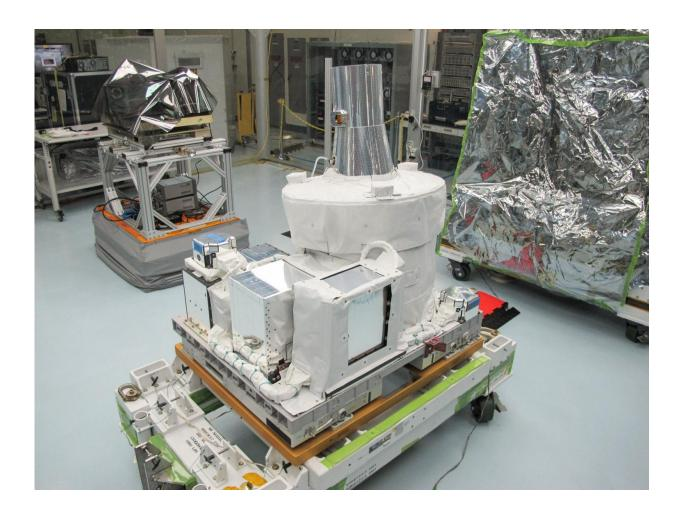
The SAGE III instrument integrated on the EXPRESS Pallet Adapter (ExPA) after its final sharp edge inspection before its launch on Space X 10. This investigation will measure the stratospheric ozone, aerosols, and other trace gases by locking onto the sun or moon and scanning a thin profile of the atmosphere. Credit: NASA
