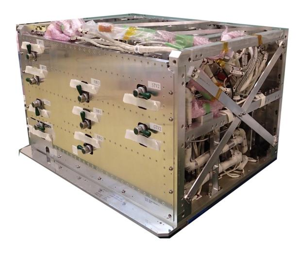
The experiment hardware, which installs in the Multi-purpose Small Payload Rack in the KIBO module of the space station. Credit: JAXA
