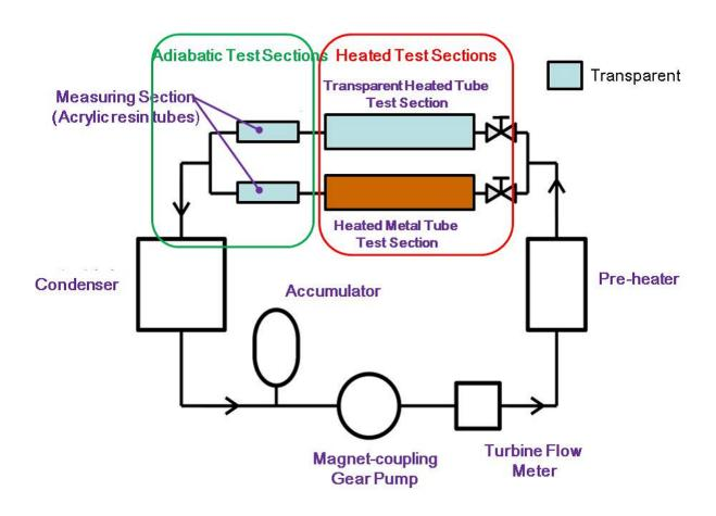
Schematic diagram of test loop for flow boiling. Credit: JAXA
