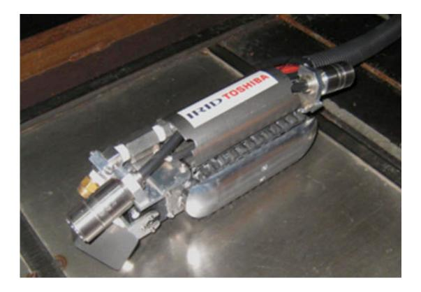
This undated photo released by Tokyo Electric Power Co. (TEPCO) shows a remote-controlled "cleaning" robot which is to be used for inspection inside the reactor containment chamber of Unit 2 at Fukushima Dai-ichi nuclear power plant. The "cleaning" robot that entered one of three tsunami-wrecked Fukushima reactor containment chambers on Thursday, Feb. 9, 2017, was withdrawn before completing its mission due to glitches most likely caused by high radiation. (TEPCO via AP Photo)
