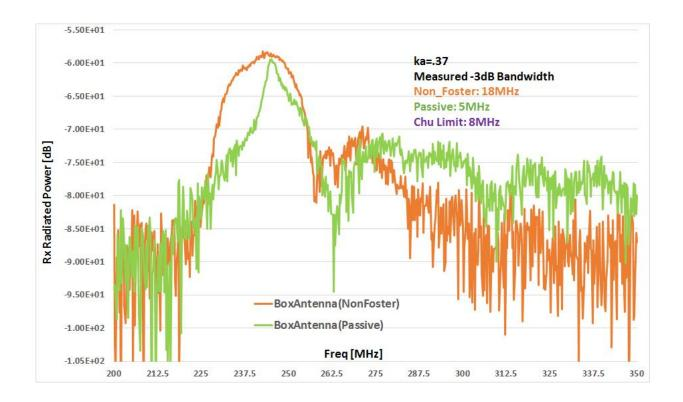
Measured bandwidth performance comparison of non-Foster integrated antenna vs. passive (conventional) antenna of the same physical size. Credit: Space and Naval Warfare Systems Center
