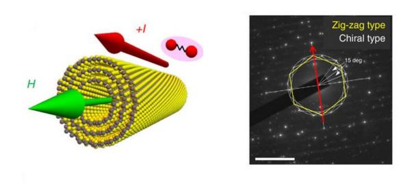
When a magnetic field is applied parallel to a superconducting chiral nanotube, electric signals travel in one direction only. (Left) Illustration and (right) electron diffraction pattern of a single tungsten disulfide nanotube. Credit: Qin et al. Nature Communications
