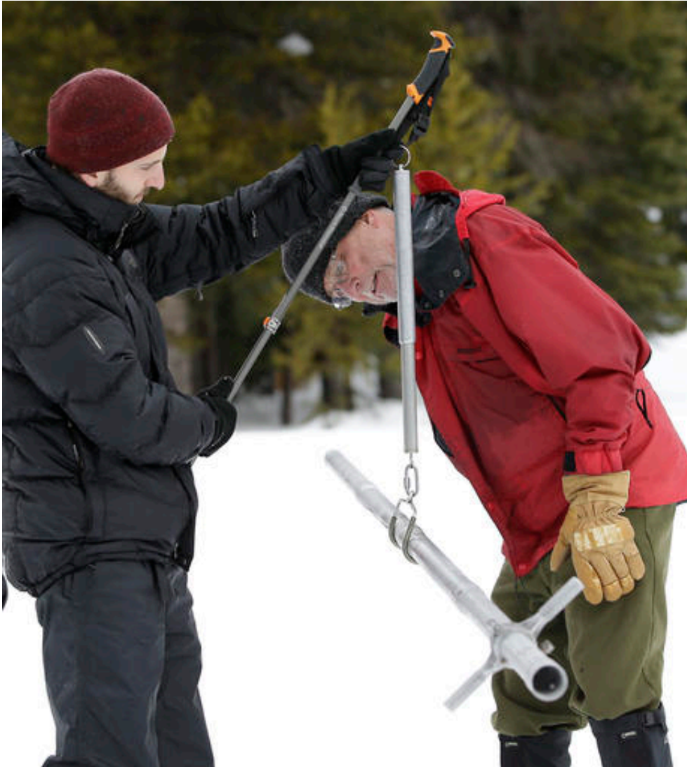
Frank Gehrke, right, chief of the California Cooperative Snow Surveys Program for the Department of Water Resources, checks the weight of the snow sample on a scale held by Mikel Shybut, a policy fellow with the California Council on Science and Technology, during the second manual snow survey of the season at Phillips Station Thursday, Feb. 2, 2017, near Echo Summit, Calif. (AP Photo/Rich Pedroncelli)
