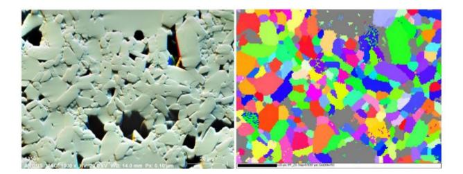
This image for Sandia National Laboratories' Brittle Materials Assurance Prediction Program illustrates the microstructure of a brittle material as seen through a scanning electron microscope, left, and a graphic showing the grain orientation of that microstructure. Credit: Sandia National Laboratories
