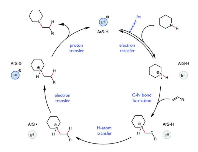
Proposed catalytic cycle for hydroamination. Credit: (c) *Science* (2017). DOI: 10.1126/science.aal3010
