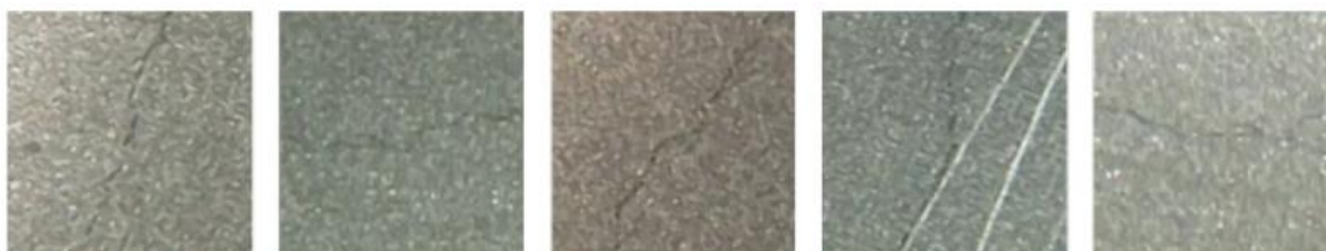
(a) Tiny cracks with low contrast and different brightness.
