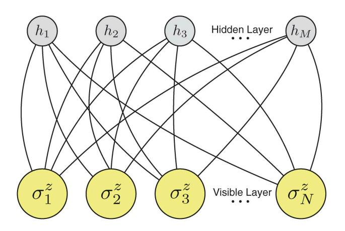
Artificial neural network encoding a many-body quantum state of N spins. Credit: (c) *Science* 10 Feb 2017: vol. 355, Issue 6325, pp. 602-606
