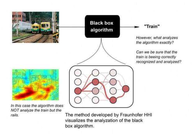
Fraunhofer HHI's analysis software uses algorithms to visualize complex learning processes (schematic diagram). Credit: Fraunhofer HHI
