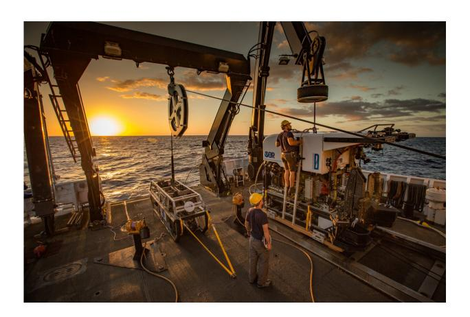
The dual-body ROV is dedicated to the ship and includes the camera sled Seirios (left) and ROV Deep Discoverer (right). Both vehicles are outfitted with powerful lighting, high-definition imaging, and sensors to collect in situ environmental information on habitats being explored. Deep Discoverer is also equipped with a temperature probe, and two manipulator arms, coral cutters, and storage boxes for sample collections. Credit: NOAA Office of Ocean
