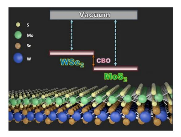
The Anderson model enables a simple way of predicting the offset of the top of the bandgap (labelled as CBO) of 2D semiconductors, such as tungsten diselenide and molybdenum disulfide. Credit: KAUST Ming-Hui Chiu
