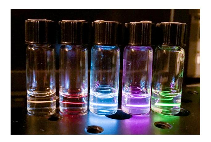
In the Dionne lab at Stanford, a laser causes nanoparticles suspended in cyclohexane to emit light. The nanoparticles change color depending on the pressure around them and give real-time information about the forces they undergo. Credit: Alice Lay
